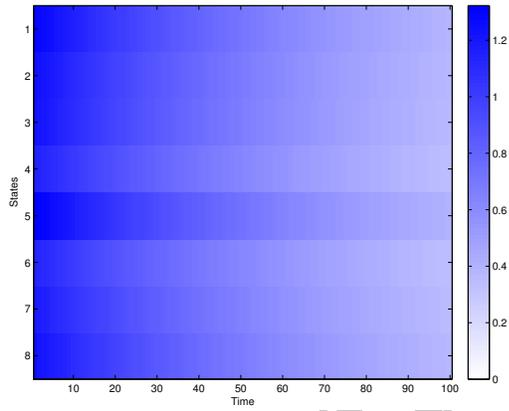
Figure 5: Impulse response of the reduced order model.
